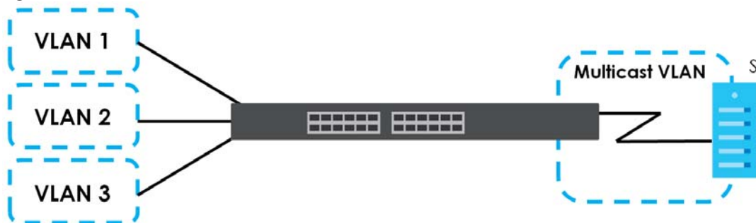
Figure 201 MVR Network Example
