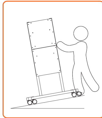
Stay above cart when moving down slope
