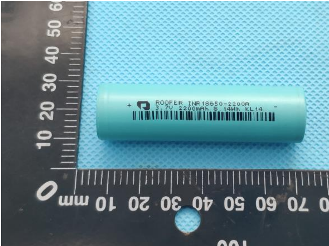
Cells /电芯 (INR18650-2200A 3.7V 2200mAh 8.14Wh)
