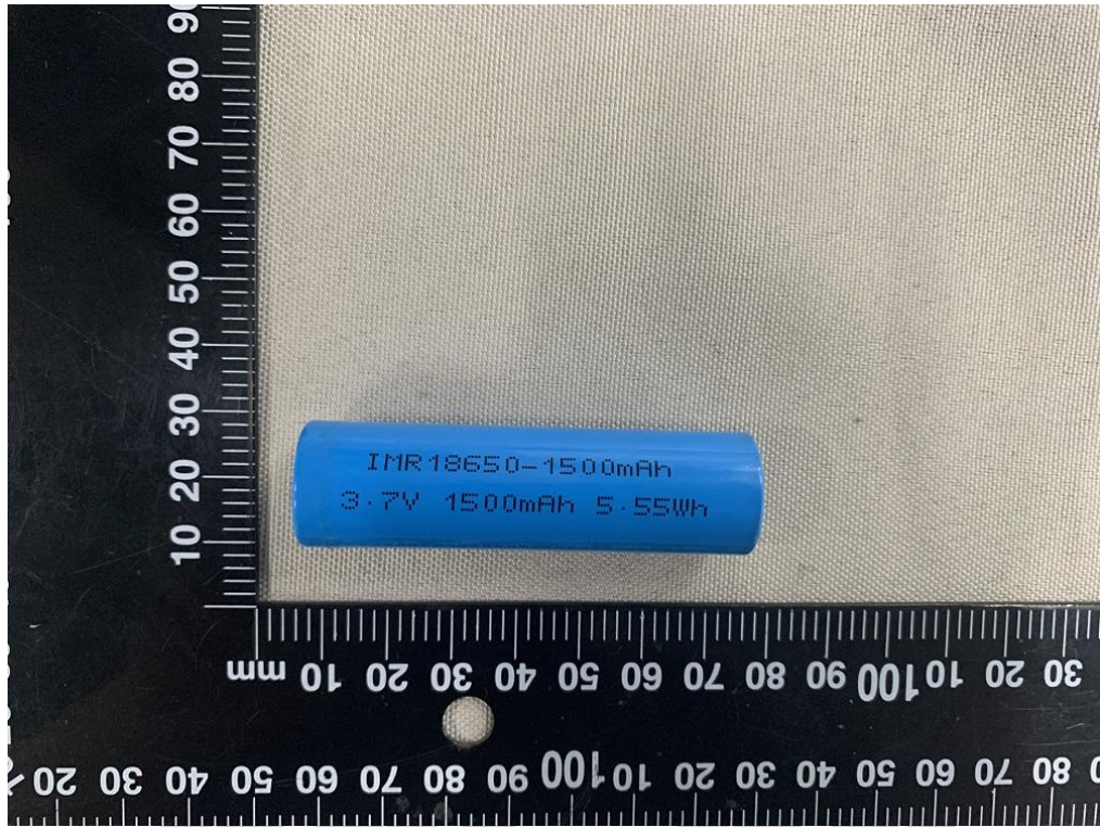
Cell (IMR18650-1500mAh, 3.7V, 1500mAh, 5.55Wh)
