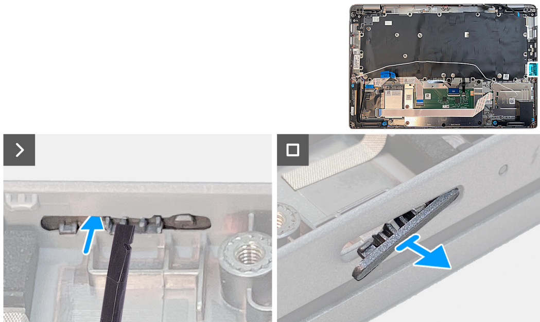
Figure 65. Removing the dummy SIM-card slot filler
