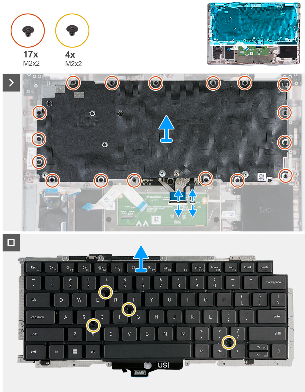
Figure 61. Removing the keyboard
