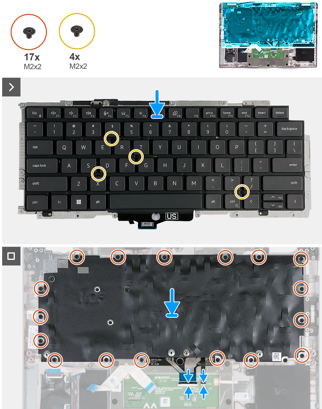
Figure 62. Installing the keyboard
