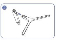
Remove the stand neck from the stand base by pulling it in the direction of the arrow as shown in the figure.
