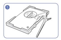
Place the protective Styrofoam (cushion) included in the package on the floor and place the product facing down on the Styrofoam, as shown in the image. If Styrofoam is unavailable, use a thick sitting mat.
