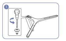
Turn the connecting screw at the bottom of the stand base to separate it.
