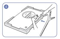
Hold the back of the product as shown in the figure. Push the assembled stand into the main body in the direction of the arrow as shown in the figure.
