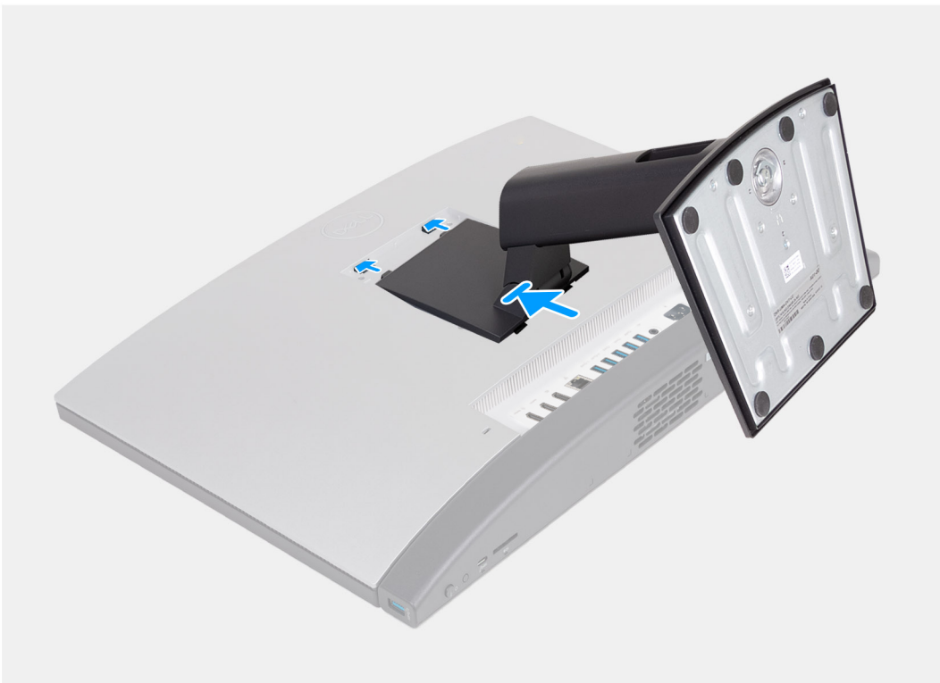
Figure 18. Installing the Fixed Stand
