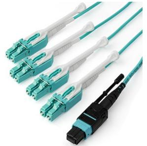
This MPO/MTP to 4x LC breakout cable lets you fan out a single 40Gbps connection from a 40GBase-SR4 QSFP+ transceiver to four 10Gbps LC SFP+ transceivers.
