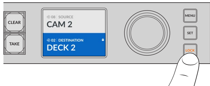
To prevent routes from being switched on a specific output, press the lock button to lock the output
