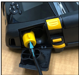
1. Insert connector in communications port.
