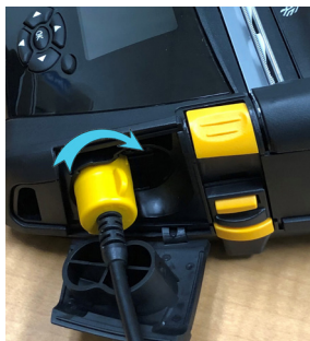
2. Rotate locking cap clockwise to secure.
