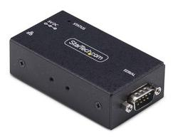
This serial-to-IP converter is an efficient solution for remotely connecting and controlling a variety of RS232 serial devices over an IP-based network.
