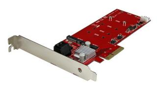
This M.2 SSD RAID controller card lets you install two M.2 NGFF (Next Generation Form Factor) drives in your desktop computer. The card also features two SATA III (6Gbps) ports and supports hardware RAID. Now, you can merge the speed and compact size of M.2 solid state drives (SSD) with the storage capacity of traditional hard disk drives (HDD).
