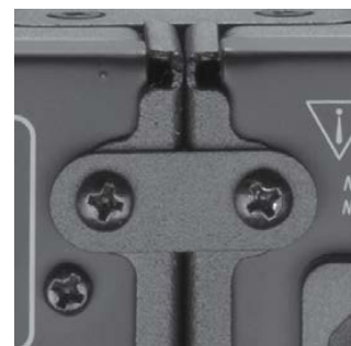
Figure 6. Install Back Plates (2 places)
