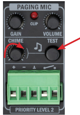
Figure 12. Paging Mic Adjustments
