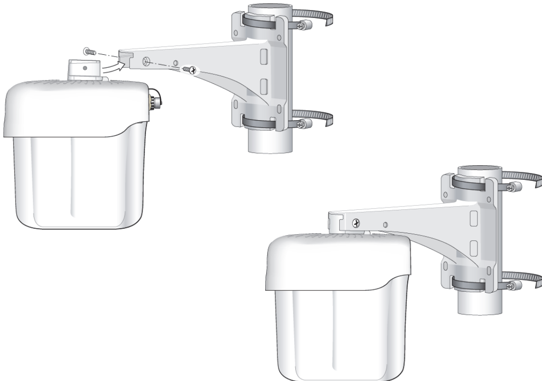
Figure 6 Attaching the AP to the Mounting Bracket
