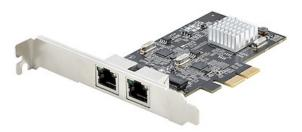
This dual-port 2.5GbE network interface card (NIC) features independent Intel I225-V chipsets for each port with Intel vPro technology, to enhance performance and data integrity across two 2.5G ethernet connections. The variable multispeed options (2.5/1Gbps and 100/10Mbps) enable support for both new and legacy network hardware. Utilize existing Cat5e or CAT6 cabling infrastructure while adding NBASE-T (802.3bz) compatibility for seamless integration.
