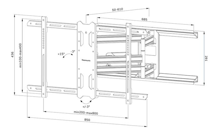
Neomounts Measuring unit: mm
