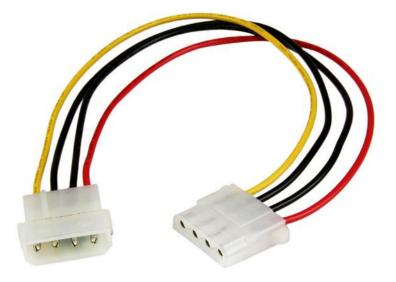
The LP4POWEXT12 Extension Cable features two 4-pin lp4 power connectors, one male and one female, and offers 12-inches in cable length, enabling you to extend your LP4 power connections and allowing you to position your devices (i.e. hard drive, DVD-ROM drive, add-in card, etc.) as needed within the system case.
