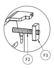
ii. Slide item F1 down the front slots of item D1 to the correct height and tighten items F2.
