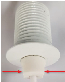
Figure 8 Pinch-Points for Microphone Cable Length Adjustment
