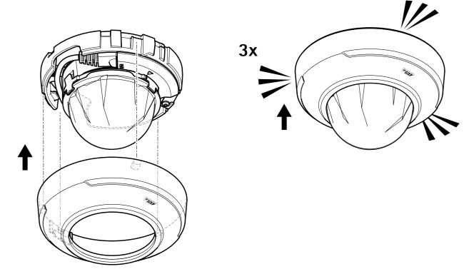
1. Line up the dome cover to the dome and snap the two parts together (3 snaps).
