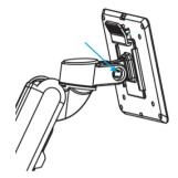
To increase / decrease swivel resistance, adjust the set screws located beneath the swivel points using a Phillips screwdriver, or on the base of the arm using the 3mm Allen Wrench (5).
