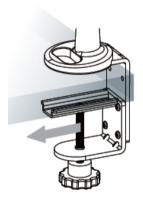
**Note:** The Desk Clamp can support a desk / table thickness from  $\frac{3}{4}$  - 3.94 in (20 – 100 mm). Depending on the thickness of your desk / table, the clamp can be adjusted smaller by removing the 4 screws and raising the bottom portion of the clamp as shown below.
