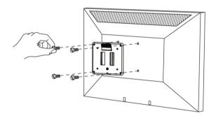
**Warning:** Do not over-tighten the screws and stop immediately if you encounter resistance to avoid damage to your display. Ensure that all screws being used are the same length and thread type.
