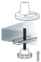
5. Slide the Monitor Arm (1) onto the base and tighten the set screw on the back of the base, using the 3mm Allen Wrench (5).
