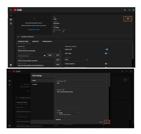
5. Users can see the Stream Key and Stream URL that are provided by the Youtube streaming platform. Please copy the stream key and stream URL and then paste them into the "First Stream MRL" within the "Network" option of the PTC-280 Web UI. Please click "On" and please check the checkboxes of "Audio" and "Video".
