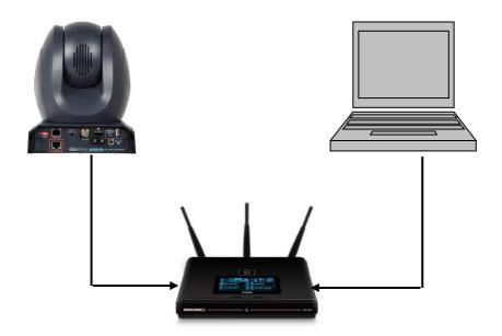
In order to enable the DHCP mode of the camera, please select "Dynamic IP Address" from the "IP Configuration Type" drop-down menu for assigning a dynamic IP address to PTC-280 by the router. After that, please click the "Apply" button to save the new settings and then please reboot the PTC-280.
