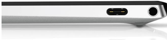
Figure 1: Thunderbolt 4 laptops with an 11th Generation Intel-Core processor may be missing the Thunderbolt logo.
