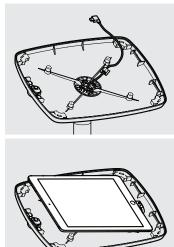
7 Install the tablet into the Case & connect to power.
