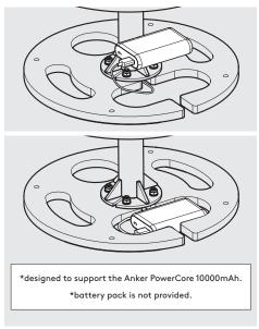
**9.2** If installing a battery pack, connect the tablet cable and locate the pack into the Floorstanding Base.
