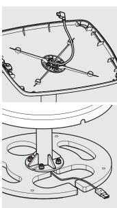
Feed the tablet power cable through the Case & Floorstanding Pole.
