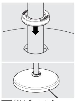
With the Floorstanding Cover on the ground, locate and fit the Floorstanding Rubber Collar.
