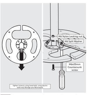
Orientate, locate and secure the Floorstanding Pole to the Floorstanding Base as shown. Ensure that all fixings are installed correctly.
