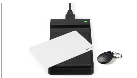
USB reader for RFID cards and fobs
