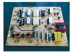
S23-1 Cut the glue between bulk cap. and PCB with a knife.
