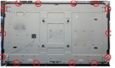
Disconnect the touch cable and FFC cables. Use a screwdriver to remove13pcs screws(Torque: 6±0.3kgf), 12pcs screws (Torque: 3±0.3kgf) for unlocking the
