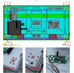
Take 1pcs rear cover, assemble the rear cover with the assembled unit, then use a screwdriver to lock the rear cover with 60pcs screws.(Torque: 3±0.3kgf) Assemble 4pcs handles with the rear cover, then lock the handles with 16pcs screws.(Torque:15±0.5kgf)
