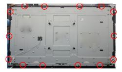
Disconnect the touch cable and FFC cables. Use a screwdriver to remove13pcs screws(Torque: 6±0.3kgf), 12pcs screws (Torque: 3±0.3kgf) for unlocking the ED holder with the assembled unit.
