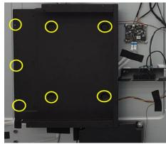
Remove the handles and rear cover, then remove the 5pcs rubbers as the picture below shown.
