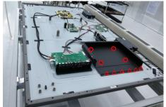
Paste 2pcs rubbers on the specific positions of topside, and then paste 2pcs rubbers on the specific positions of bottom-side. Paste 1pcs rubber on the side of driver board as the picture below shown.
