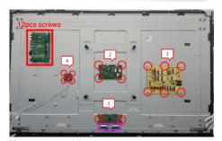
Use a screwdriver to remove 42pcs screws
