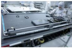
Use a screwdriver to remove 24pcs screws for unlocking the bottom-middle bezel and then remove the bottom-middle bezel.(Torque: 2±0.3kgf)
