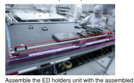
back bracket, then push the whole unit into a tripper, then fix the FFC cables with tapes, then paste 2pcs rubbers on the specific position as the picture below shown.
