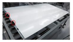
Use a sucking tool to suck 1pcs LGP, then tear off the protective film of the LGP. Assemble the LGP with the Reflector and back bracket, then power on and make sure there is no particles on the film.
