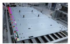
Take 1pcs touch cable to connect the ED boards as picture 1. Take 1pcs folded FFC cable to connect the ED boards as picture 2, then assemble 2pcs rubbers to the assembled unit as picture 3 and picture 4.
