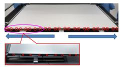
Take 1pcs bottom-ED-holder and 2pcs small brackets, then use a screwdriver to tighten 8pcs screws for locking the two bracket with the bottom ED holder.
