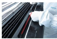
Take 1pcs light pipe, and then use a screwdriver to lock 2pcs screws for locking the light pipe with front bezel. Take 1pcs IR board and 1pcs IR holder and 1pcs shading tape, then assemble the IR board with IR holder, then use a screwdriver to lock 2pcs screws for locking the IR holder with front bezel.(Torque: 3±0.3kgf)
