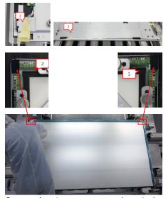
Operate the tripper to overturn the unit, then use a screwdriver to lock 10pcs screws for locking the ED unit with the back bracket, then turn over the unit for later assembling.(Torque: 3.0±0.3kgf)
