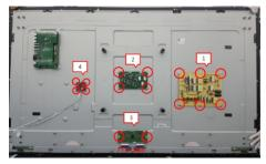
Use a screwdriver to lock 4pcs screws to the back bracket, then use a screwdriver to lock 4pcs screws for locking 1pcs main board with the screws, and then assemble 1pcs USB board and 1pcs IO holder with the main board, then lock 4pcs screws for locking the USB board, lock 4pcs hex screws for locking the VGA connectors. (Torque:4.5kgf±0.3)
