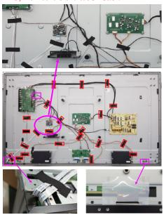
Place 1pcs PC box to the specific positions of the S34 whole unit, then use a screwdriver to lock 10pcs(4+6) screws for fixing the PC box. (Torque:3±0.3kgf)
