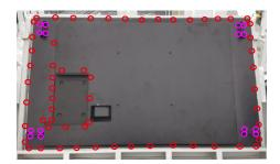
Remove the handles and rear cover, then use a screwdriver to remove 7pcs screws for releasing the PC box.(Torque: 4.5±0.3kgf)
