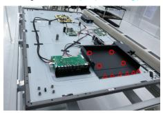
Remove 2pcs O/C mylar tapes away from the back bracket, then remove 22pcs black tapes and 1pcs conductive tape as the picture below shown.
