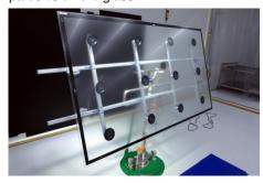
Use a sucking tool to suck the glass and then assemble the glass with the O/C module, then tear off all release papers around edges of the O/C module., and then press the glass with a roll for two parts firmly attachment.
