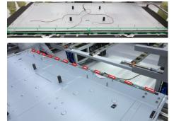
Make sure ED FFC cables are connected well, then assemble 1pcs ED holder with the assembled unit, and then use a screwdriver to tighten 13pcs screws for locking the ED holder with the assembled unit. (Torque: 6±0.3kgf)Use a screwdriver to tighten 12pcs screws for locking the ED holder with the unit. (Torque: 3±0.3kgf)
