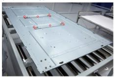
Tear off the papers of the tapes on the L/B heat sink, then assemble the L/B heat sink with back bracket.
