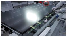
Use the tapes to fix the SB of the O/C on the back bracket, then use the tipper to turn over the unit to let the back bracket faced up.
