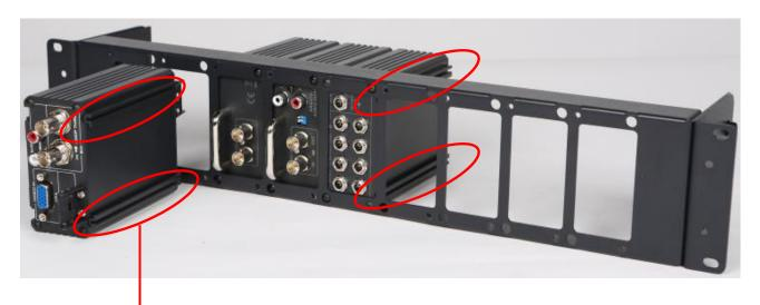
When attaching your devices to the RMK-2, please make sure all devices are aligned as shown in the above diagram.
