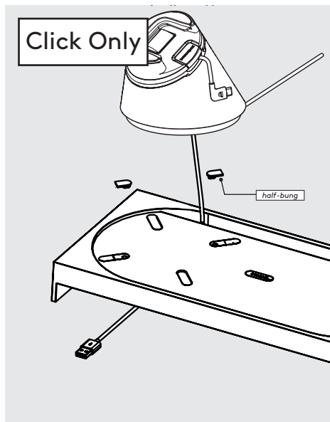
9 Lift up the Click Stand and remove the INNER half-bungs from Caddy.
