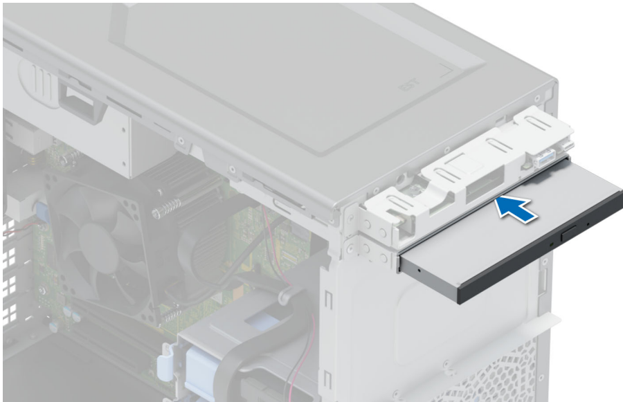
Figure 27. Installing the optical drive
