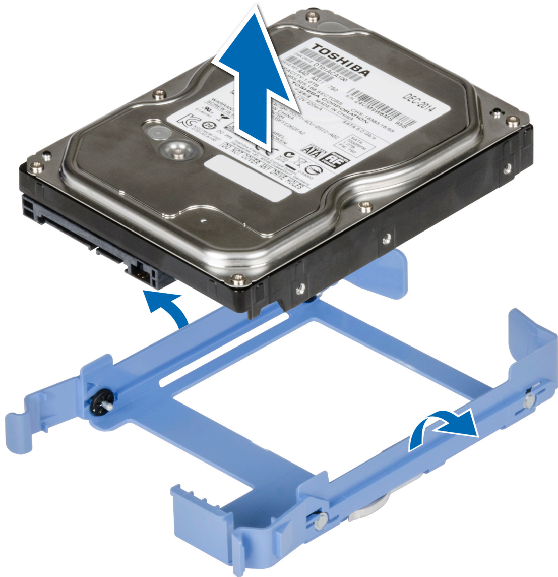
Figure 14. Removing the drive from the drive carrier
