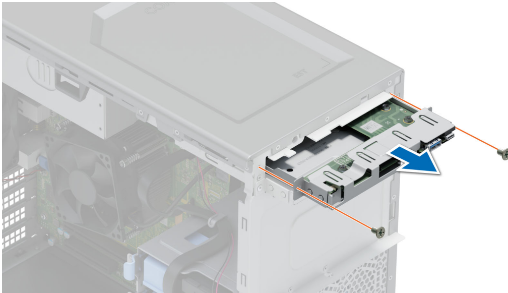
Figure 59. Removing the control panel cage
