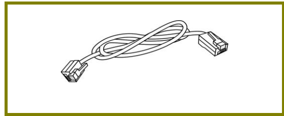
RJ-11 to RJ-11 Cable (Annex A) (Connects to your DSL line)
