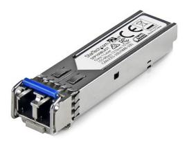
The SFP100BLXST is an MSA compliant fiber SFP transceiver that's designed, programmed and tested to work with 100BASE-LX compatible MSA switches and routers. The SFP transceiver module supports a maximum distance of up to 10 km (6.2 mi) and delivers dependable 100 Mb Ethernet connectivity over fiber cabling. <br/>
