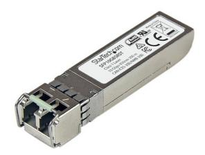
The SFP10GBSRST is an MSA compliant fiber SFP transceiver that's designed, programmed and tested to work with 10GBASE-SR compatible MSA switches and routers. The SFP+ transceiver module supports a maximum distance of up to 300 m (984 ft) and delivers dependable 10 GbE connectivity over fiber cabling.
