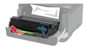
**Warning—Potential Damage:** Do not expose the imaging unit to direct light for more than 10 minutes. Extended exposure to light may cause print quality problems.
