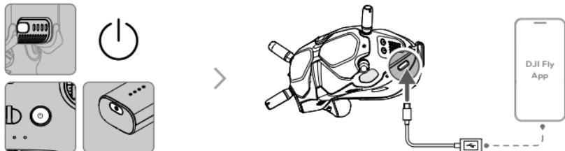
Connect the USB-C port of the goggles to the mobile device, run DJI Fly, and follow the prompt to activate.
