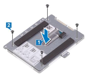
3 Connect the interposer to the hard-drive assembly.
