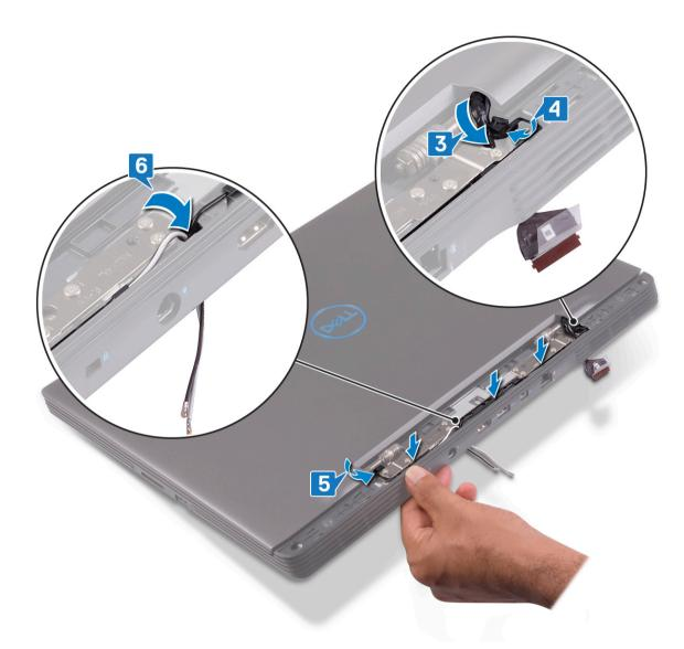
7 Align the hinge cover with the slots on the palm-rest and keyboard assembly and press to secure the hinge cover to the palm-rest and keyboard assembly.
