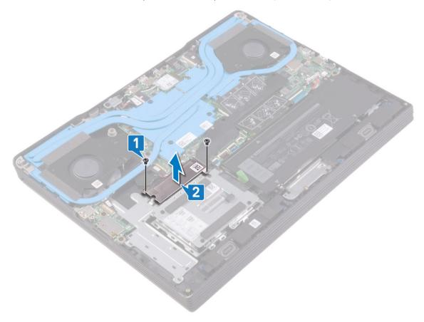
3 Remove the screw (M2x4) that secures the solid-state drive/Intel Optane to the palm-rest and keyboard assembly.
