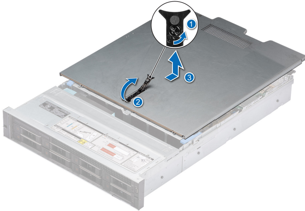
Figure 20. Removing the system cover
