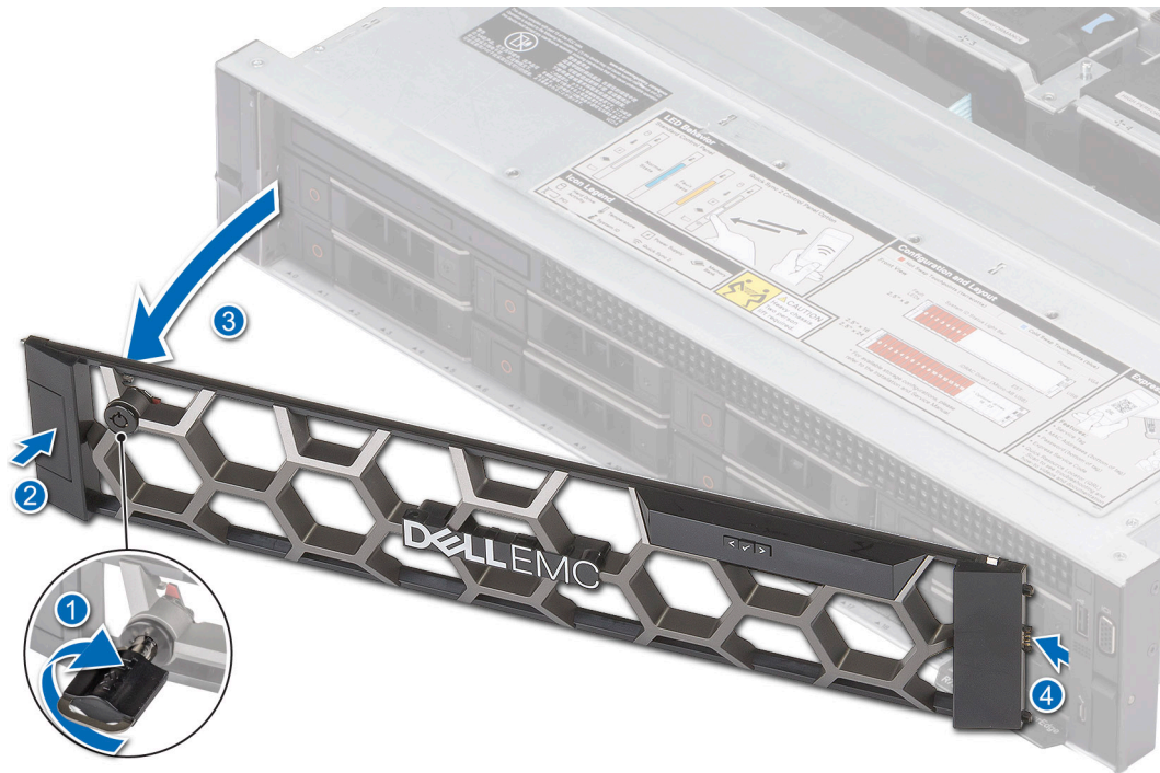
Figure 18. Removing the front bezel with the LCD panel
