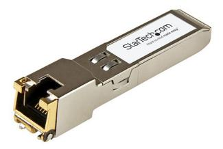
The CG-ST is a Palo Alto Networks PAN-SFP-CG compatible copper transceiver module that has been designed, programmed and tested to work with Palo Alto Networks brand switches and routers. It delivers dependable 1 GbE connectivity over copper cable, for 1000BASE-TX compliant networks, with a maximum distance of up to 100 m (328 ft).
