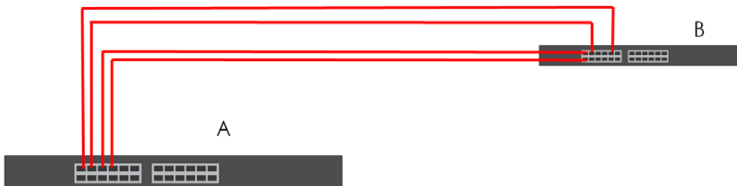
Figure 164 Trunking Example – Physical Connections
