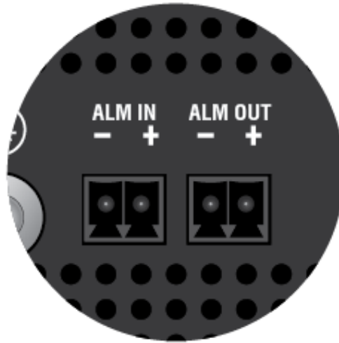
Figure 38. Polarity Legend for the Alarm Connectors
