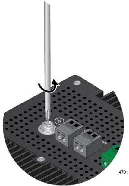
Figure 35. Loosening the Grounding Screw
