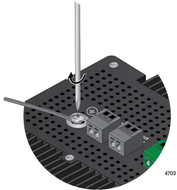
Figure 37. Securing the Grounding Wire to the Switch
