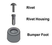
Figure 23. Parts of the Bumper Feet
