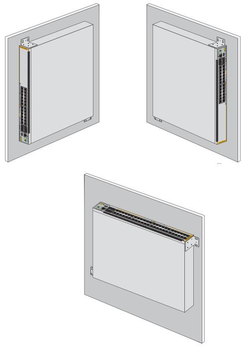
Figure 32. Positioning the AT-x530L-28GTX or AT-x530L-52GTX Switch on the Wall
