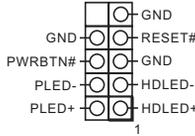
Connect the power switch, reset switch and system status indicator on the chassis to this header according to the pin assignments below. Note the positive and negative pins before connecting the cables.
