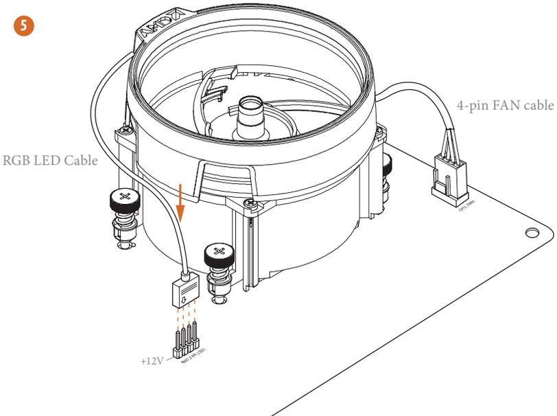
\*The diagram shown here are for reference only. Please refer to page 34 for the orientation of AMD Fan LED Header (AMD\_FAN\_LED1).
