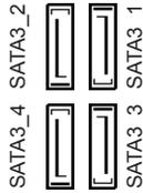
These four SATA3 connectors support SATA data cables for internal storage devices with up to 6.0 Gb/s data transfer rate.
