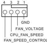
This motherboard provides a 4-Pin CPU fan (Quiet Fan) connector. If you plan to connect a 3-Pin CPU fan, please connect it to Pin 1-3.
