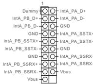
There is one header on this motherboard. Each USB 3.1 Gen1 header can support two ports.
