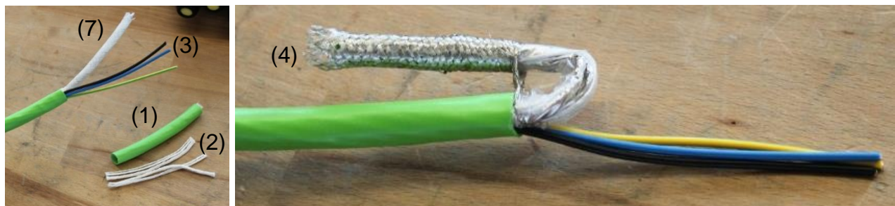
Figure 2.2 – Stripped cable and bare shielding
