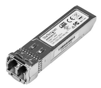
The 455883B21ST is a TAA compliant HPE 455883-B21 compatible fiber transceiver module that has been designed, programmed and tested to work with HPE brand switches and routers. It delivers dependable 10 GbE connectivity over fiber cable, for 10GBASE-SR compliant networks, with a maximum distance of up to 300 m (984 ft).
